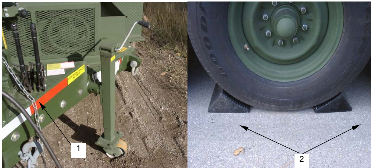
Figure 5. Trailer Leveling and Wheels Chocked
