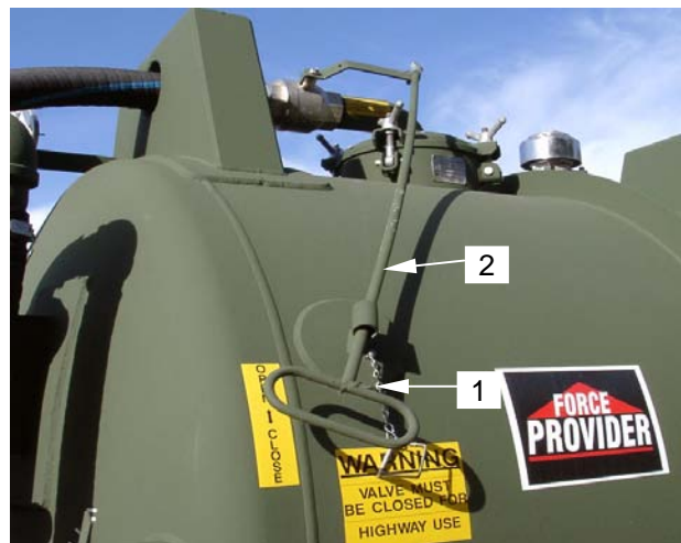
Figure 16. Isolation Valve Control
