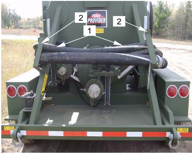
Figure 12. Removing 2 ½-inch Hoses
