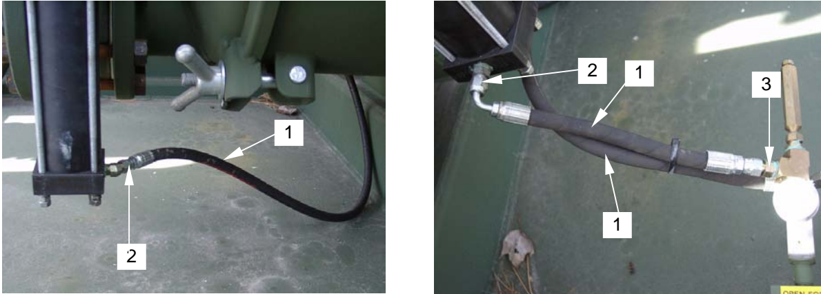
Figure 2. Replacing Hydraulic Hoses
